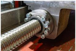
Classic recirculating ball screw: although the mechanical linear drive is efficient and accurate, it must be rigidly connected to an electric motor, and the force it can exert is limited.
