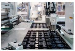
ATAM's automated coil encapsulation and testing
